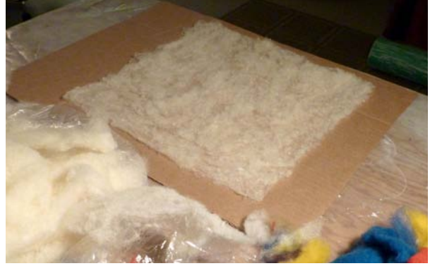
2 wool is first arranged in approximately two to three very thin layers that alternate direction of the fibers
